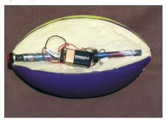
Fig. 2. Cutaway of the Doppler Football. This ball was destroyed so we could photograph the internal arrangement.
