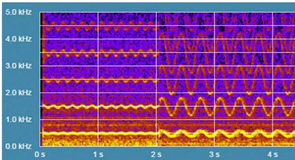
**Figure 3.** Frequency modulation.
