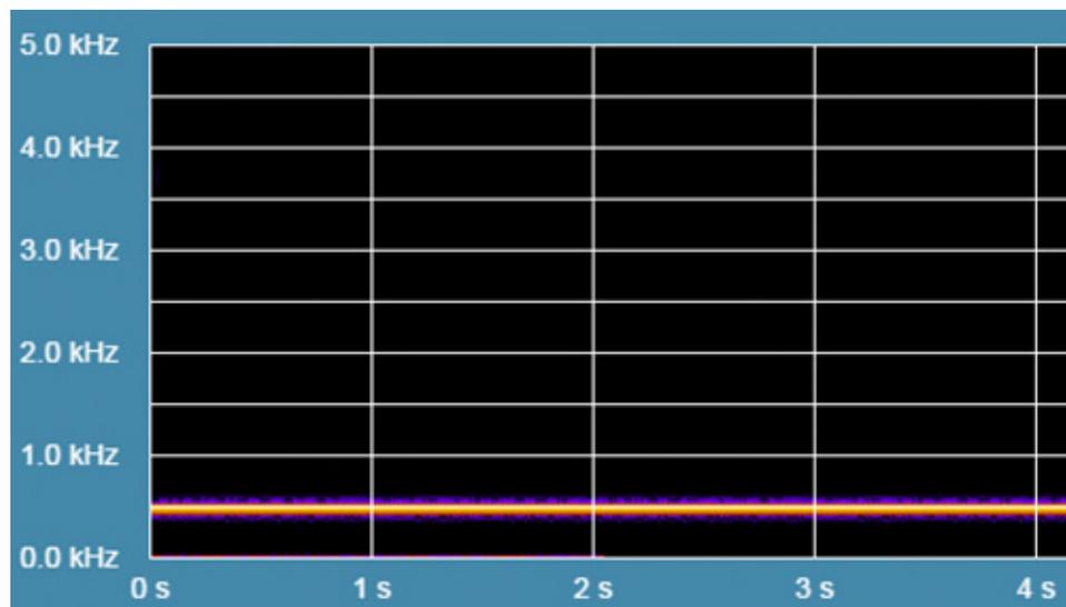
**Figure 1.** Spectrogram of a 500 Hz sine wave.
