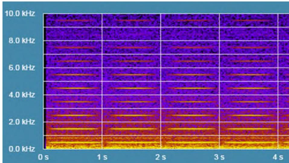
**Figure 2.** A 500 Hz square wave undergoing amplitude modulation.
