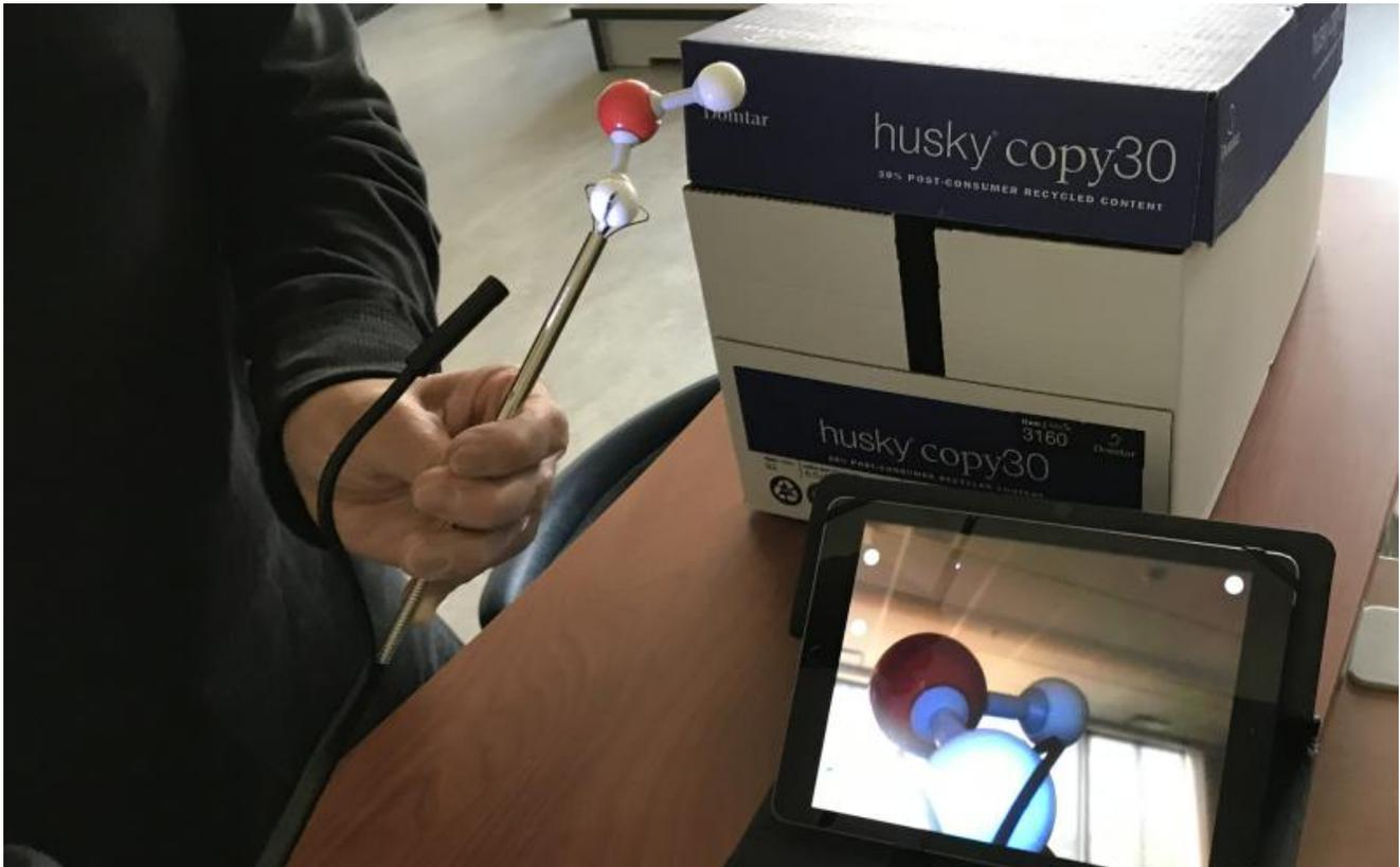
**Figure 3.** Endoscope and grabber holding water molecule with Bluetooth image transmitted to the iPad. Note that the endoscope has been pulled up near the grabber to make viewing and navigation easier.
