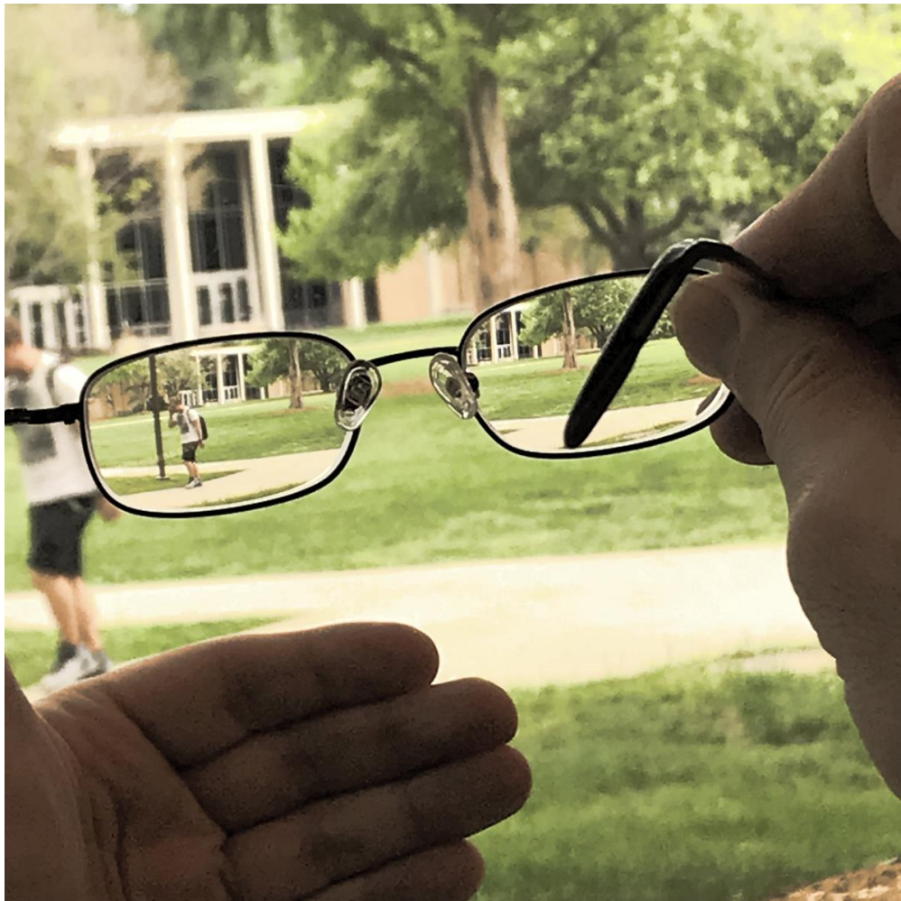
Figure 3. Eyeglasses where each lens is -5D . Distant images have corresponding virtual images in the plane at a distance of 20 cm from the lens, in which plane the left hand is also located.
