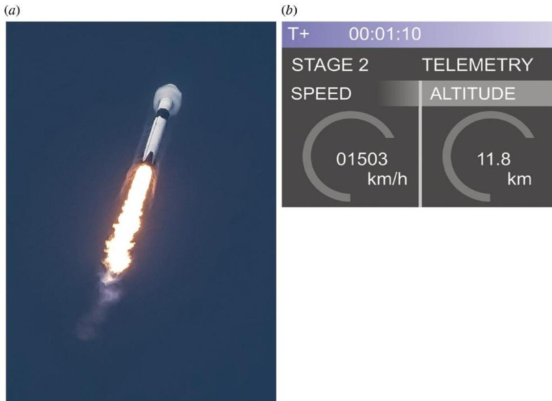
**Figure 4.** (a) Photo of the Falcon 9 carrying the Bangabandhu satellite into space, 11 May 2018. Reproduced with permission from [5]. (b) Sample telemetry data that appears in a section of the SpaceX videos. The telemetry data changes in real time, matching the speed and altitude of the spacecraft.
