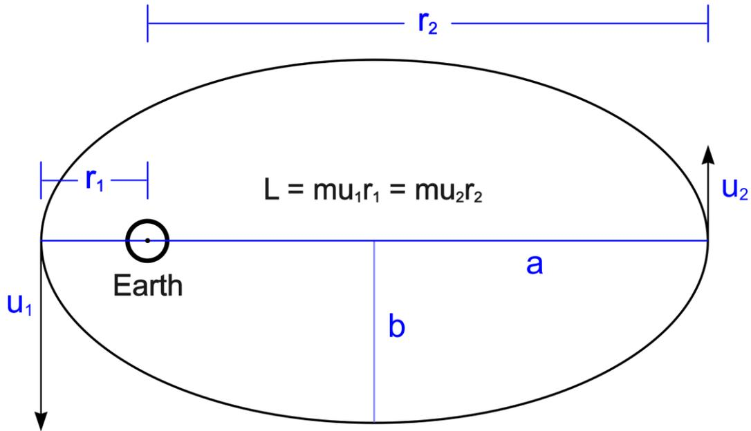
**Figure 3.** A satellite in an elliptical orbit around the Earth with semi-major axis  $a$  and semi-minor axis  $b$ . The angular momentum  $L$  takes on a simple form at the extreme orbital points since the velocity vector is perpendicular to the radial vector at each of the extreme points.
