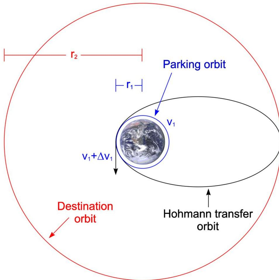
**Figure 2.** Parking orbit, Hohmann transfer orbit, and destination orbit. Earth image is Public Domain Courtesy NASA. Actual view of Earth would be looking down at the North Pole for a geostationary destination orbit.
