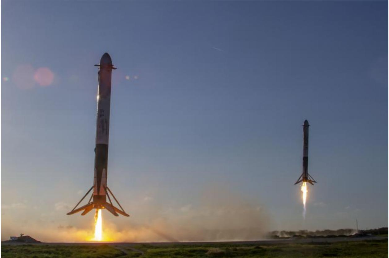
**Figure 6.** Two rocket boosters of the Falcon Heavy landing after use. Reproduced with permission from [5].
