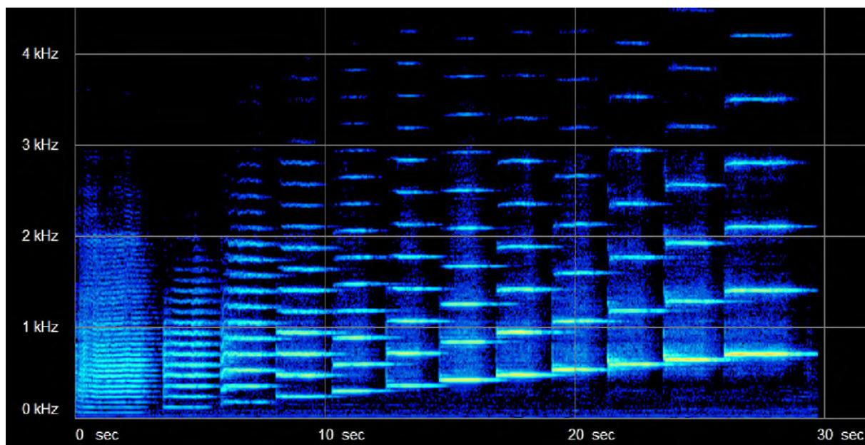
**Figure 5.** Spectrogram of the first 12 tones of the French horn harmonics beginning on  $B_1^b = 58.3$  Hz . The PC desktop app is *Spectrogram 16* by Richard S. Horne.
