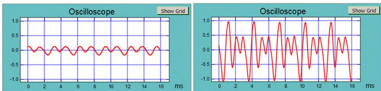
**Figure 1.** Oscilloscope view of a soft tone (left) and one for a loud tone (right).
