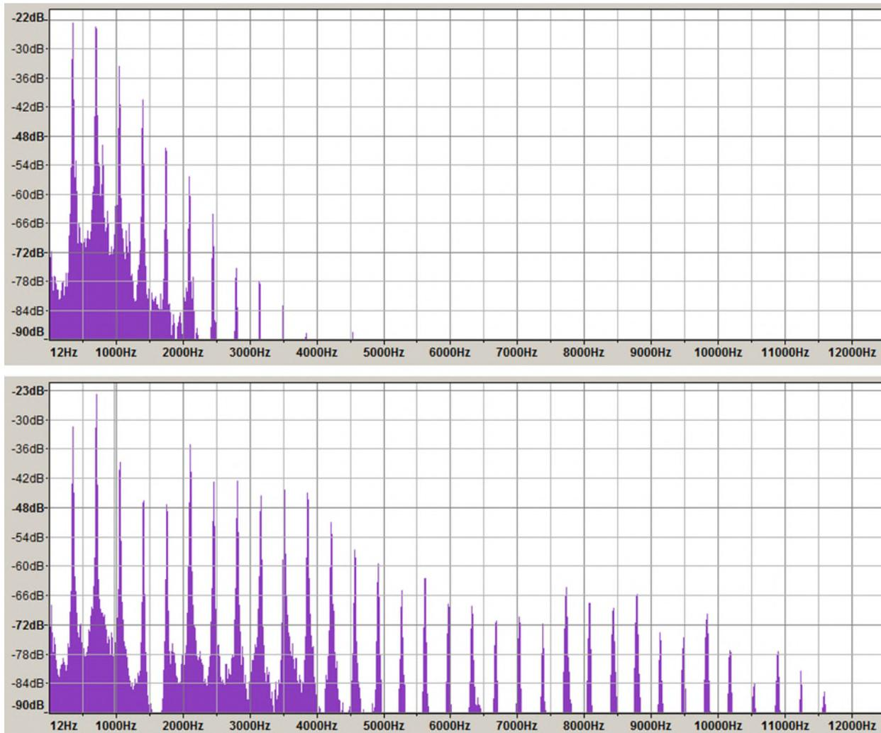
**Figure 8.** Strengths of partials against their harmonic frequencies for the normal tone of the French horn (top) and the sound produced when the right hand is inserted significantly into the bell.
