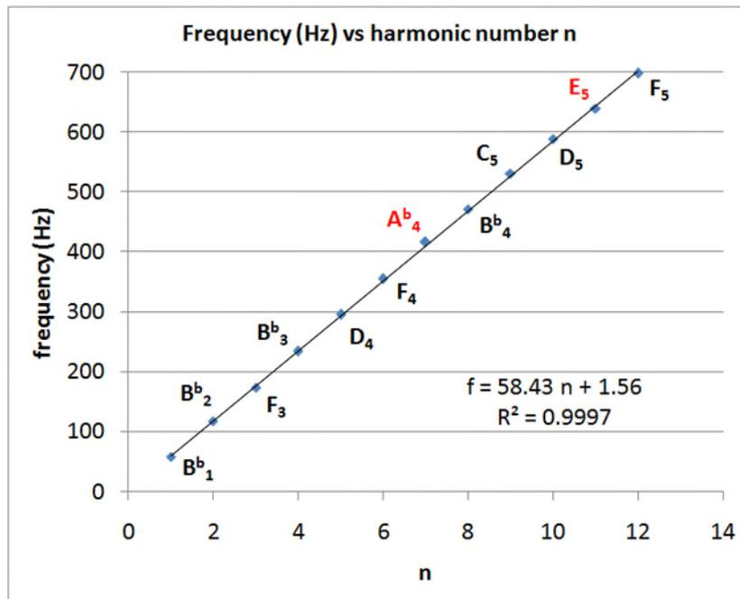
**Figure 4.** Measured frequencies of the French horn harmonic series starting on  $B_1^b = 58.3$  Hz . The red indicates that the harmonic is slightly out of tune when compared to its corresponding concert pitch. The experimental value is  $B_1^b = 58$  Hz from the slope of the linear fit.
