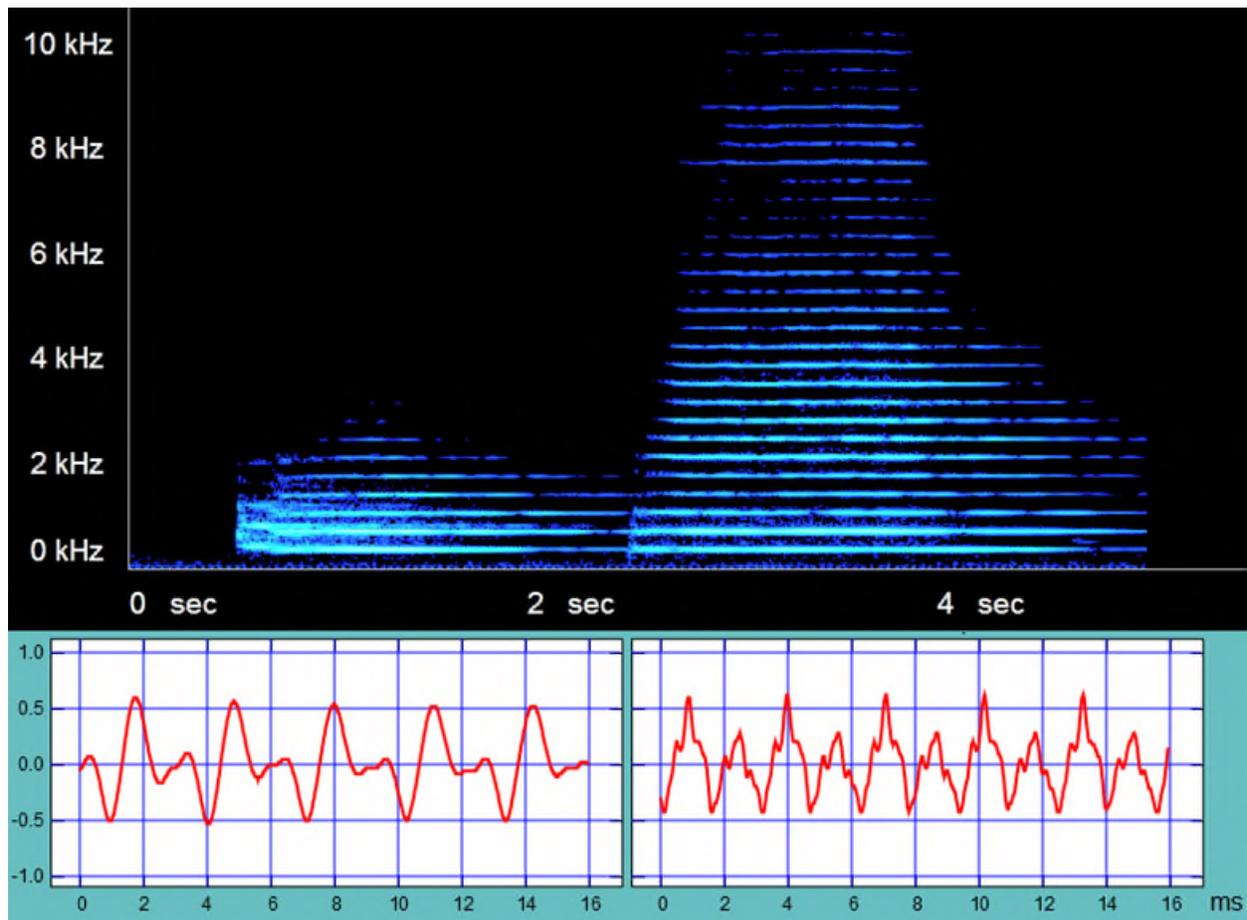
**Figure 7.** Spectrogram and oscilloscope waveform for normal playing (left) and playing with the right hand deeply inserted into the bell (right). Note the drastic change in timbre (waveform) appearing on the oscilloscope and the addition of many partials for the richer wave on the right.
